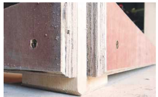
▲ Pic.4 Between the jointed cross rail is a free rail (here being hammered) and some roofing batten to make up the gap. Too many joints would have weakened the very area I was trying to strengthen. These pieces were then cut out for the vices and copiously screwed to each other
